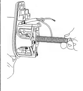
Assembling carbon brushes Use suitable tool to lift springs and insert carbon brushes. Pay attention to installation position mark. Use spring balance to check brush contact force. Spring balance
